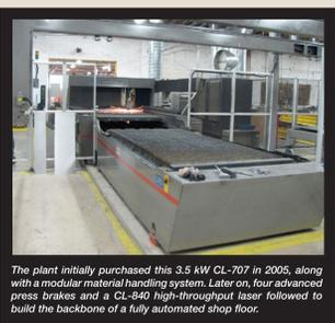
The plant initially purchased this 3.5 kW CL-707 in 2005, along with a modular material handling system. Later on, four advanced press brakes and a CL-840 high-throughput laser followed to build the backbone of a fully automated shop floor.
