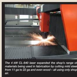
The 4 kW CL-840 laser expanded the shop’s range of materials being used in fabrication by cutting mild steel from 11 ga to 22 ga and even wood – all using only shop air.
