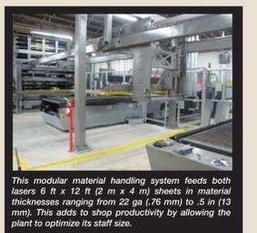
This modular material handling system feeds both lasers 6 ft x 12 ft (2 m x 4 m) sheets in material thicknesses ranging from 22 ga (.76 mm) to .5 in (13 mm). This adds to shop productivity by allowing the plant to optimize its staff size.
