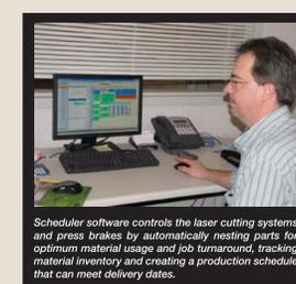
Scheduler software controls the laser cutting systems and press brakes by automatically nesting parts for optimum material usage and job turnaround, tracking material inventory and creating a production schedule that can meet delivery dates.
